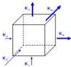
**Figure 3:** Marking of flow directions and their referring calculation planes of permeability coefficient - horizontal  $K_h$  and vertical  $K_v$
