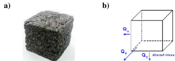
**Figure 2:** Sample of research material [10]: a) 20 x 20 x 20 mm porous material, b) diagram of the gas flow through the sample
