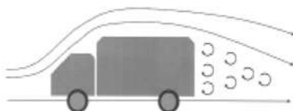
Figure 9.2. Back of the vehicle (shape with a larger negative pressure)
