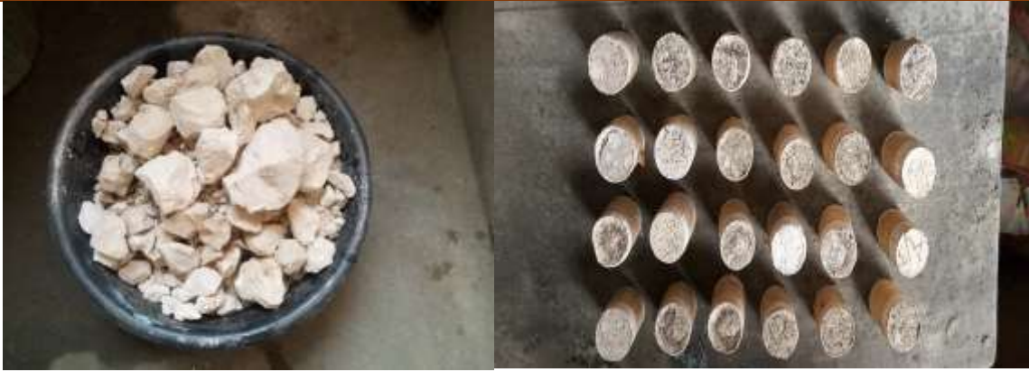
Fig 1. Shown samples of the solid raw clay directly from the site and fired samples used for characterization.
